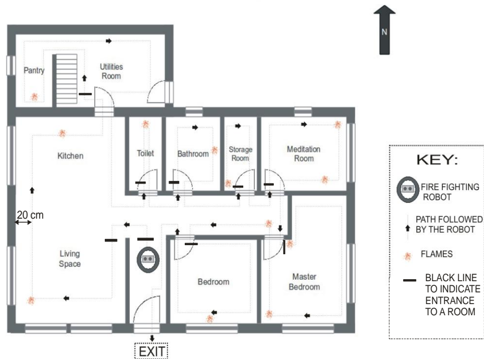
Fig. 4 Top view of the working of the fire dousing robot in a normal household (schematic)
