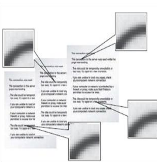
Fig. 1. Digitized books usually present recurrent patterns across different pages and across regions of the same page.
