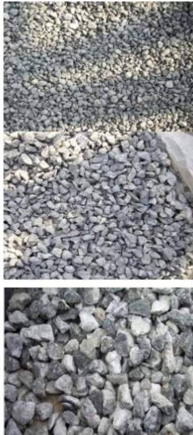
Figure 2 pictorial views of blue metal stone in various sizes of 6, 12, 20mm
