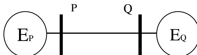
Fig.1.Transmission Line considered for analysis
