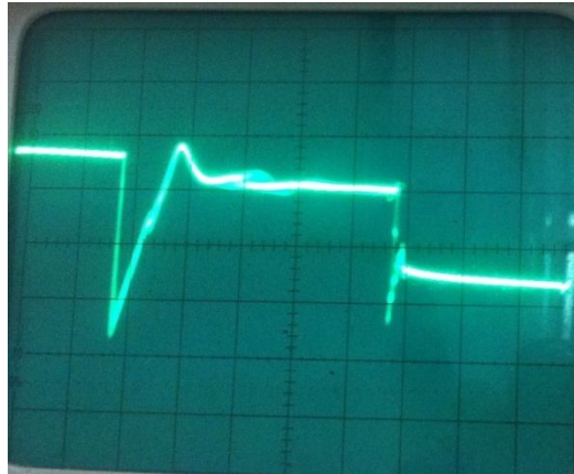
Fig 6.3 Screenshot of inverter output waveform
