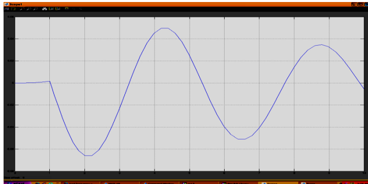
Fig.17 Frequency dynamic response of medium fast acting loops with PID Controller
