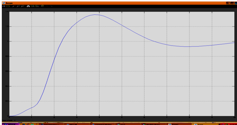
Fig.18 Dynamic response of voltage for medium fast acting loops with PID Controller
