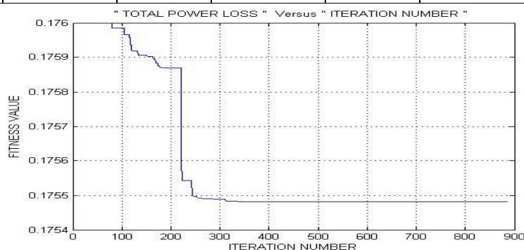
Fig 4: Performance of HSA algorithm for IEEE 30-bus system base case loading
