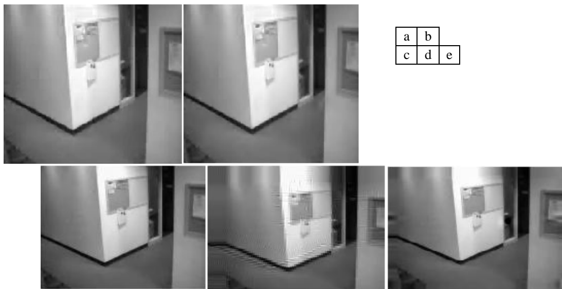
Figure.5 a) original key frame, b) compressed key frame, c)original delta frame, d)& e) are compressed delta frames using previous and proposed methods respectively of video vipmen.avi.
