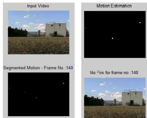
Fig. 4 Experimental output of video1 (a) Original Video files (b) Motion Estimation in video (c) Segmented motion (d) Output detection at the original video
