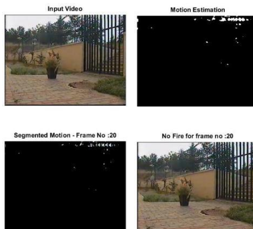
Fig. 6 Experimental output of video2-case2 (a) Original Video files (b) Motion Estimation in video (c) Segmented motion (d) Output detection at the original video
