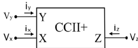
Fig1: Basic CCII+ current conveyor voltages and currents
