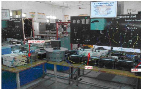
Fig.7 Lab setup of SMTB system with TCSC
