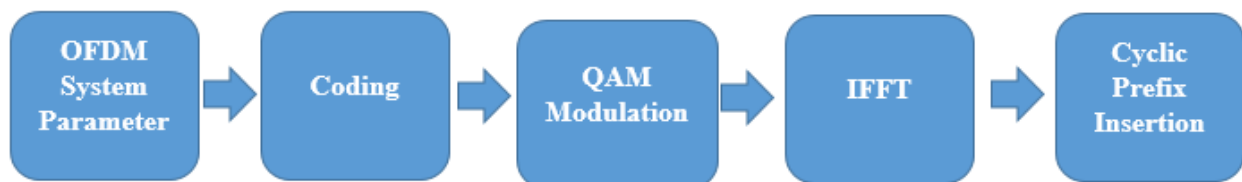
Fig.3 OFDM signal generation system [1]
