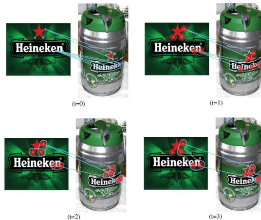
Fig. 5. Reduction of false matches with respect to the number of iterations in CDS evaluation. At t = 0 , CDS does not take into account the context and this results into the many wrong matches. As t increases, matching results become precise as the diffusion of the similarity takes into account larger and more precise context (dashed lines in figures). For ease of visualization, only a subset of interest points and their matches are shown.
