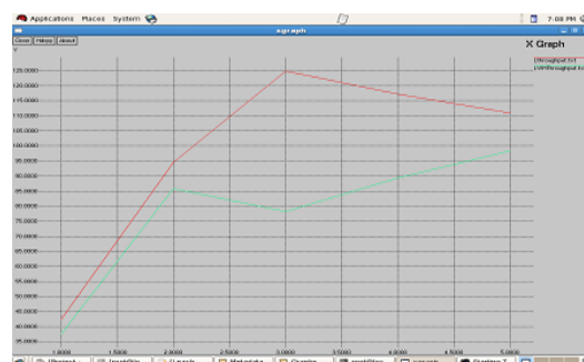
Fig. 6 LEACH Throughput with and without Wormhole
