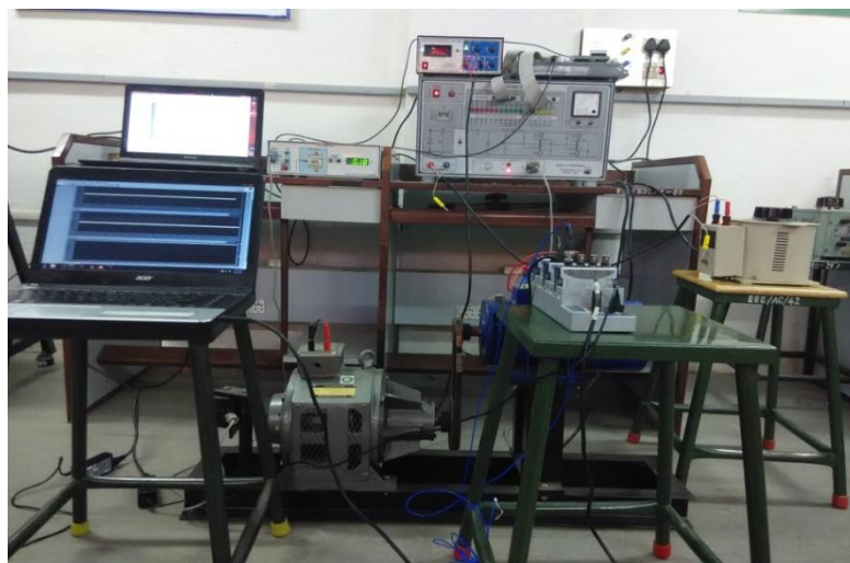
Fig.2 Experimental setup of SRM drive
