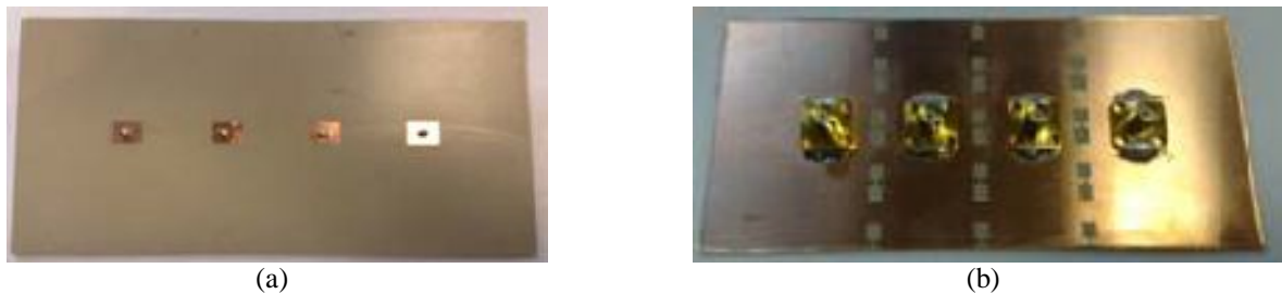
Fig. 17 Fabricated E-plane four elements linear antenna array (a) Without DGS, (b) With DGS.
