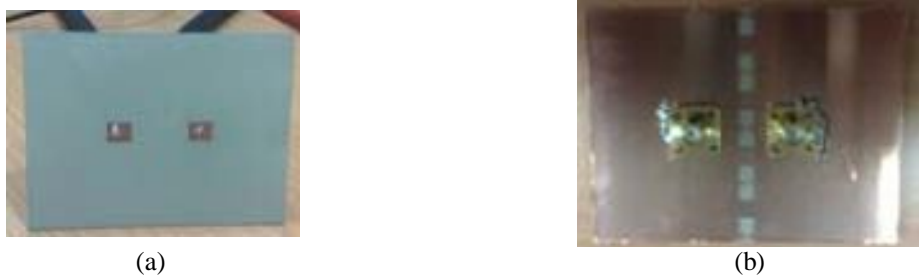
Fig. 16 Fabricated E-plane two elements antenna array (a) Without DGS, (b) With DGS.
