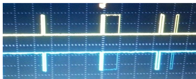
Fig 11 gating signal to the AC Chopper Switches
