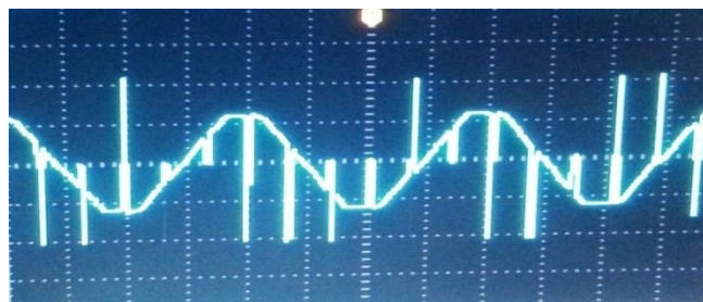
Fig 10 output voltage of Chopper
