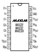
Fig: Pin diagram of MAX 232 IC SCON (serial control) register: The SCON register is an 8-bit register used to program the start bit, stop bit and data bits of data framing.
