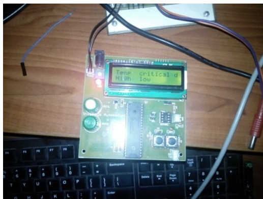
Fig.11, Temperature over alarm
