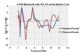
Fig 11: UWB and Bluetooth with WLAN notch Return loss
