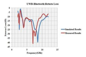
Fig 10: UWB and Bluetooth Return loss
