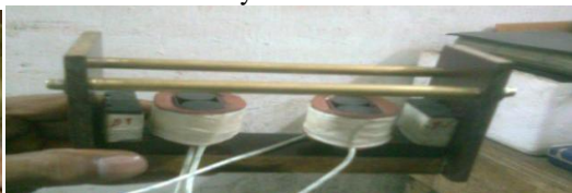
Fig 12: Ferrite core placed in the sliding unit
