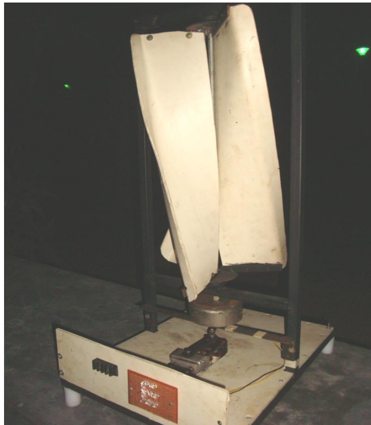
Fig 20: Over View of Vertical Axis Linear Induction (VALI) Wind Turbine
