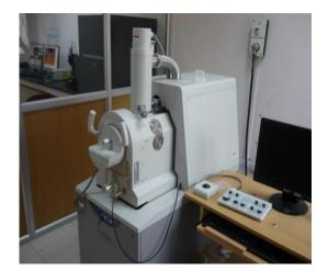
Fig. 2 Hitachi SU- 1510 Scanning Electron Microscope
