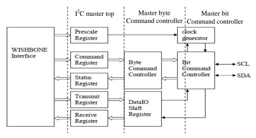
Fig 3: Components in I<sup>2</sup>C communication
