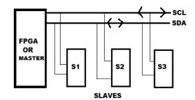
Fig 2.Master and Slave in I2C system
