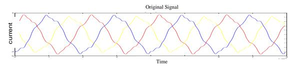
Fig.9 Current waveform for three phase induction motor under full load condition
