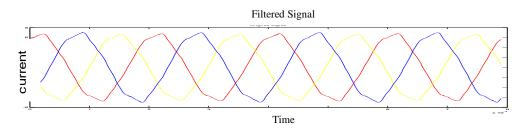
Fig.10 Current waveform with passive filter for three phase induction motor (full load)
