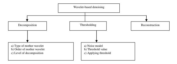
Fig.2 Wavelet-based denoising procedure
