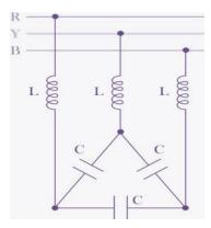
Fig.1 Typical passive filter
