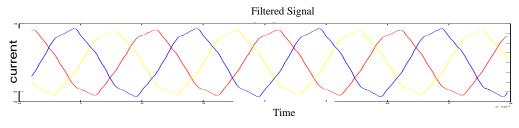
Fig. 6 Current waveform with passive filter for three phase induction motor under no load condition
