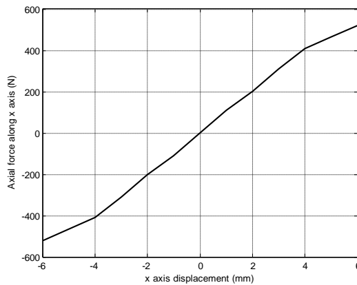
Fig. 3 Axial force Vs axial displacement (X-axis)
